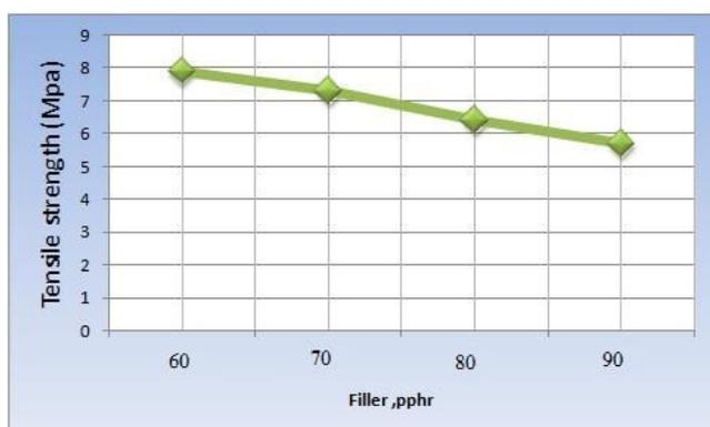
**Figure 2.** Relation between tensile strength and shells powder percentage
