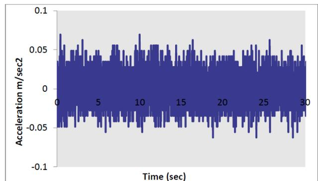
Figure 4. Time Domain Vibration Signal of the Normal Gear at 300 rpm
