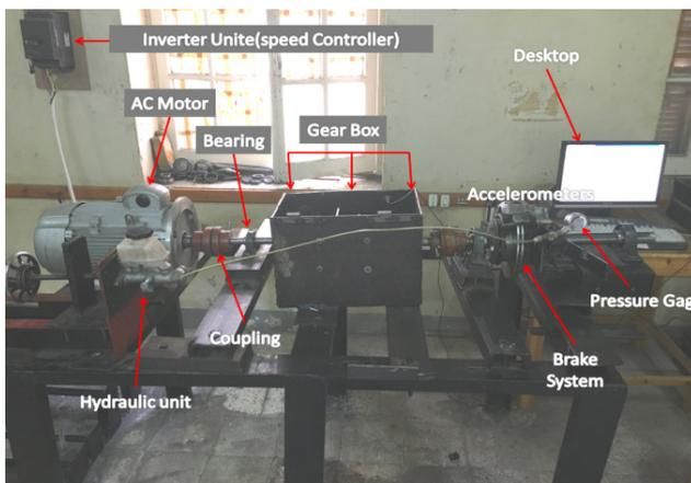
Figure 1. Gearbox fault diagnosis test rig
