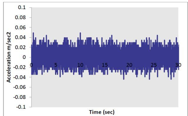
Figure 2. Time Domain Vibration Signal of the Normal Gear at 100 rpm
