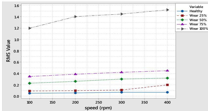
Figure 13. RMS Vibration Measurement Tooth Wear
