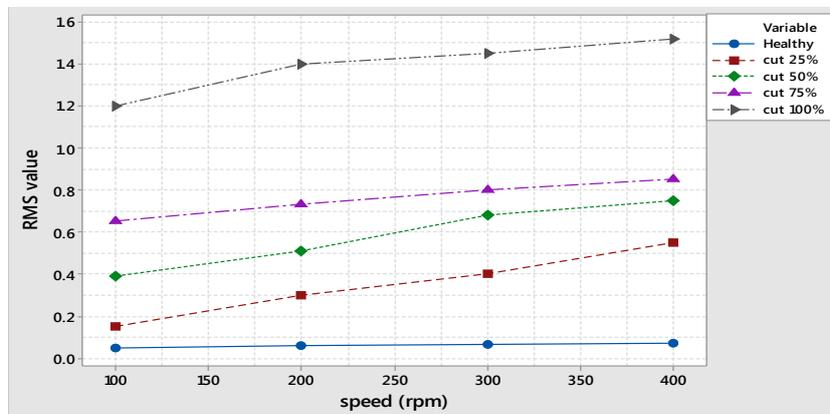
Figure 10. RMS Vibration Measurement Tooth Breakage Defect
