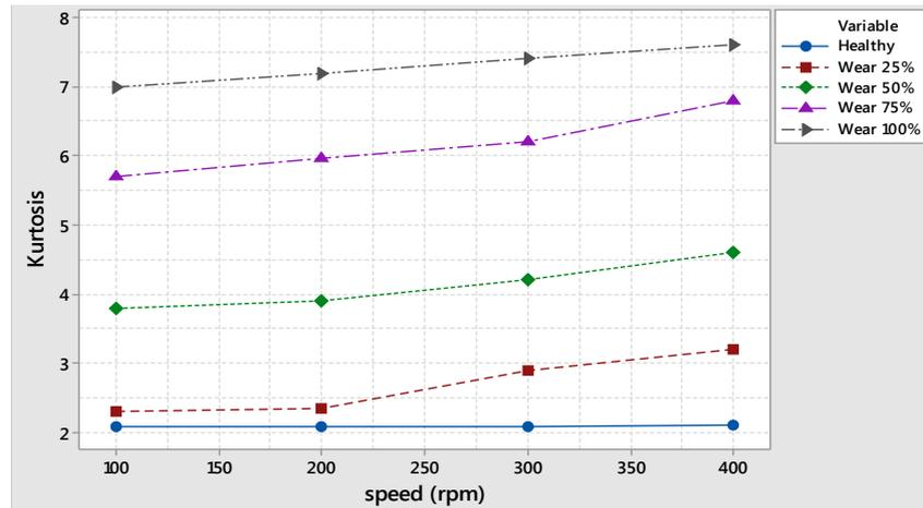
Figure 15. Kurtosis Vibration Measurement Tooth Wear
