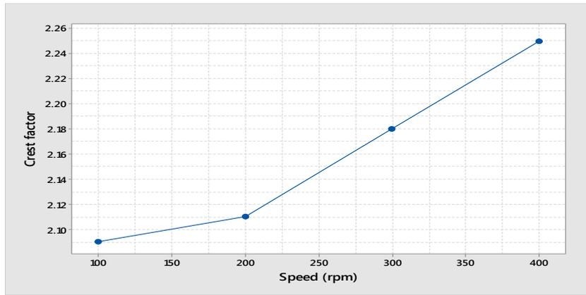
Figure 8. Crest Factor of the Normal Gear with Different Speeds
