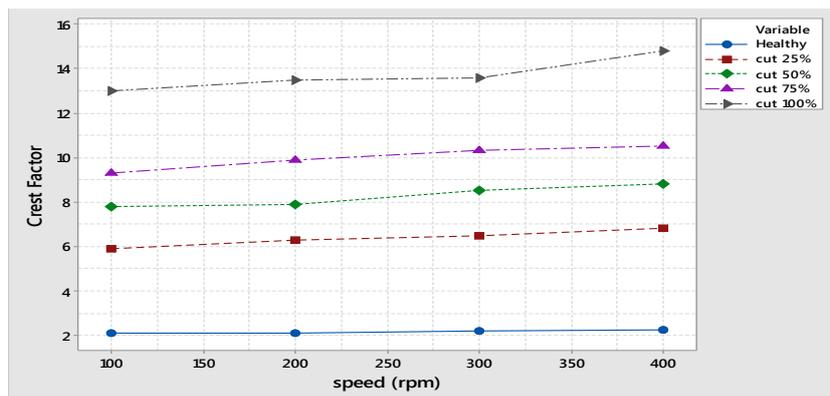
Figure 11. Crest Factor Vibration Measurement Tooth Breakage Defect
