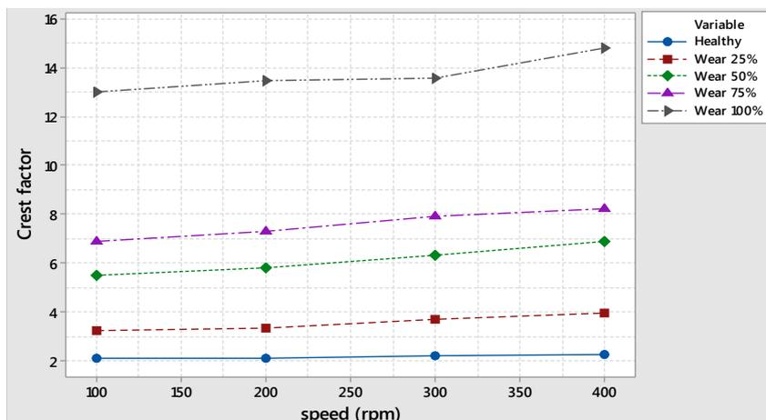
Figure 14. Crest Factor Vibration Measurement Tooth Wear
