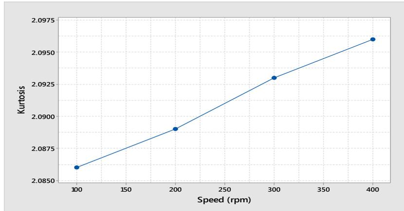
Figure 9. Kurtosis of the Normal Gear with Different Speeds
