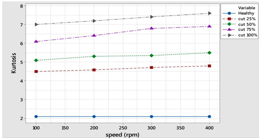
Figure 12. Kurtosis Vibration Measurement Tooth Breakage Defect
