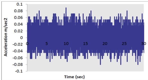
Figure 5. Time Domain Vibration Signal of the Normal Gear at 400 rpm
