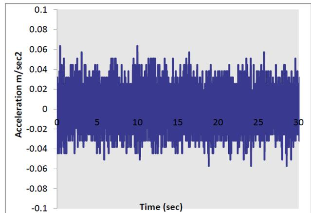
Figure 3. Time Domain Vibration Signal of the Normal Gear at 200 rpm
