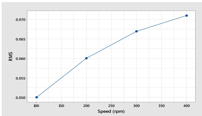
Figure 7. RMS of the Normal Gear with Different Speeds
