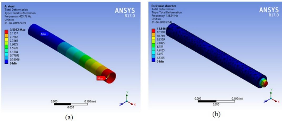
Figure 4. Cylindrical geometry ANSYS result for (a) steel layer (b) steel, foam, aluminium and gel
