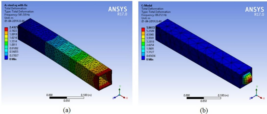
Figure 5. Square geometry ANSYS result for (a) steel layer (b) steel, foam, aluminium and gel
