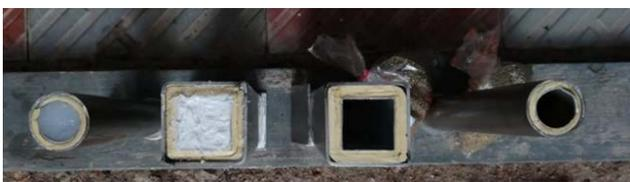
**Figure 1.** The fabricated layered shock absorbing structure with cylindrical and square geometry
