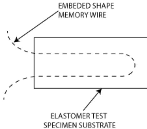
**Figure 2.** Silicone Beam with Embedded SMA wire Shaped into a Single Loop
