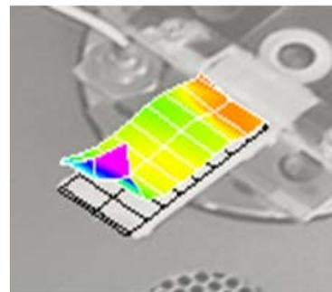
Figure 10. Mode Shape of Silicone Control Sample
