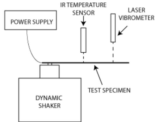
**Figure 3.** Experimental Test Setup of Silicone Beam with Embedded SMA Wire
