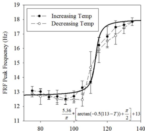
Figure 4. Graph Showing the Average Peak FRF Frequency vs. Temperature of all Eleven Runs Along with arctan Curve Fit
