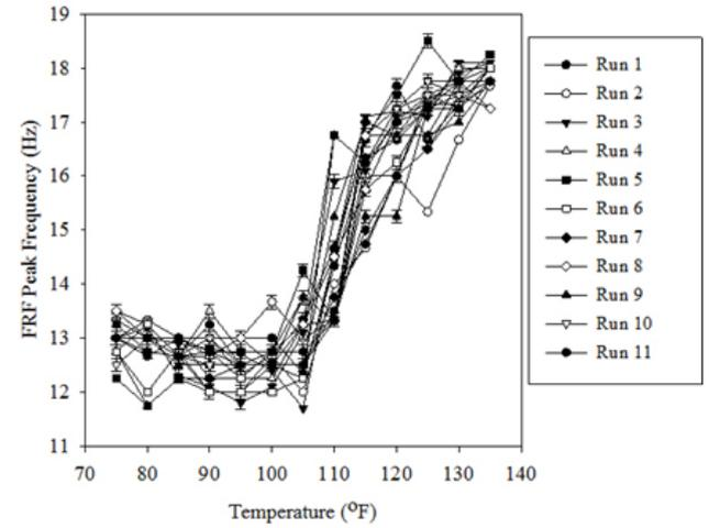
Figure 6. Graph showing Repeatability of Peak FRF Frequency vs. Temperature for Decreasing Temperatures of all Eleven Runs
