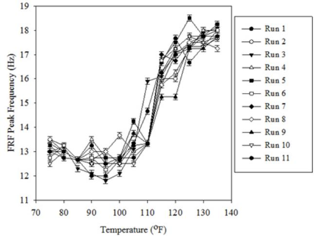
Figure 5. Graph showing Repeatability of Peak FRF Frequency vs. Temperature for Increasing Temperatures of all Eleven Runs
