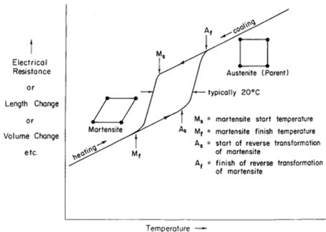
Figure 1. Theoretical plot of property change vs. temperature for the Martensite to Austenite phase transformation of a shape memory alloy [13]
