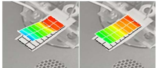
Figure 8. Mode Shape of Embedded SMA Silicone beam at 75°F (Left) and 135°F (Right)
