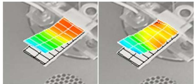
Figure 9. Mode Shape of Embedded Aluminum Silicone beam at 75°F (Left) and 135°F (Right)
