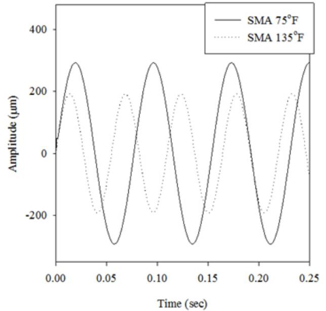
Figure 7. Maximum Tip Displacement Amplitude and Natural Frequency of Actuated and Unactuated Embedded SMA Test Sample
