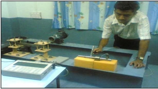
Figure 7. Photograph during the testing of Eccentric shaft on FFT analyzer
