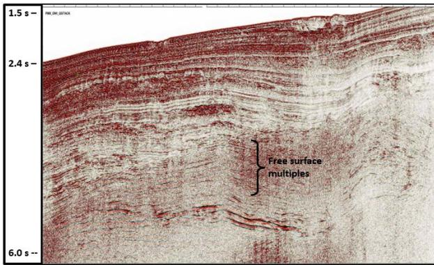
**Figure 6a.** Inline stack before 3D SRME multiple modeling and adaptive subtraction
