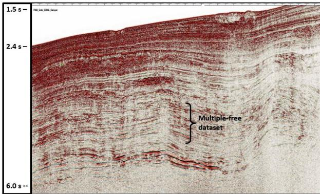
**Figure 6b.** Inline stack after 3D SRME multiple modeling and adaptive subtraction
