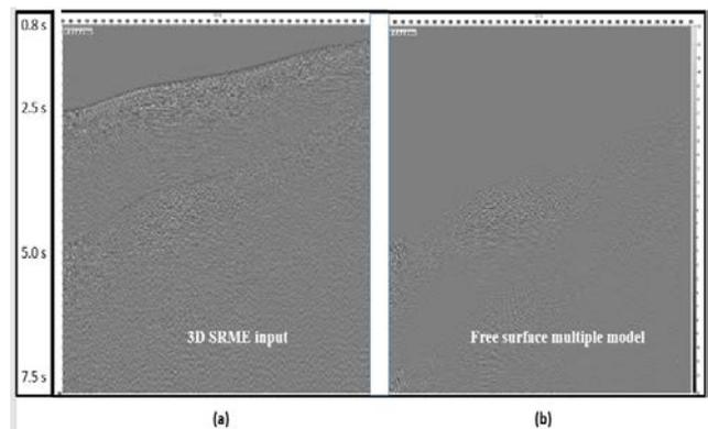
**Figure 5.** 3D multiple modeled with the parameterization in Table 2 for a test input sequence in the survey
