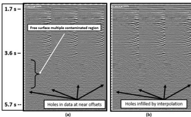
**Figure 4.** NMO-corrected, CDP track ordered input shot gathers for 3D SRME: (a) gathers before linear tau-p interpolation (b) gathers after linear tau-p interpolation
