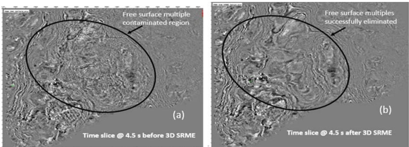
**Figure 8.** Time slice at 4.5 s showing (a) input dataset to 3D SRME and (b) post 3D SRME residual demultiple product. The displays show effectiveness of the method in attenuating free surface multiples in the dataset
