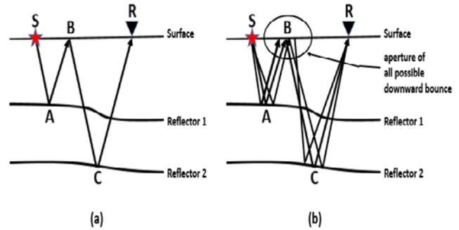
**Figure 1.** 3D SRME theory and method (a) Free surface multiple SABCR (modified from [24], in [1]) (b) and inclusion of aperture of all possible free surface multiples
