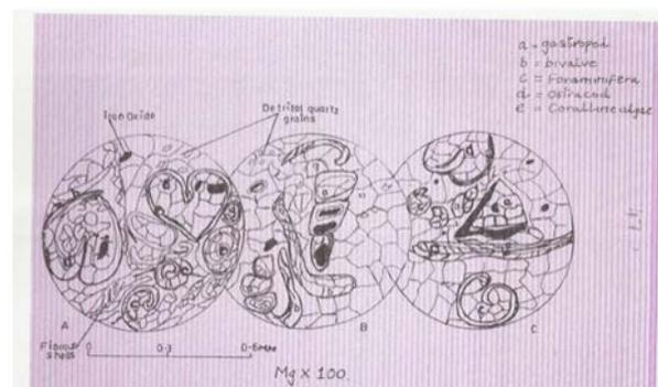
Figure 5. Thin Section Diagram of NU1 Sample under PPL
