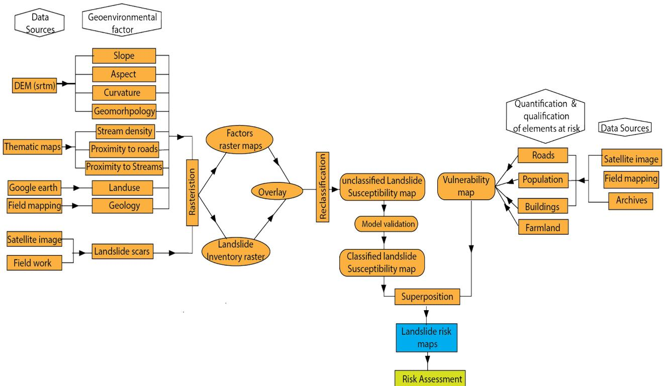
Figure 2. Landslide susceptibility mapping and risk assessment methodology
