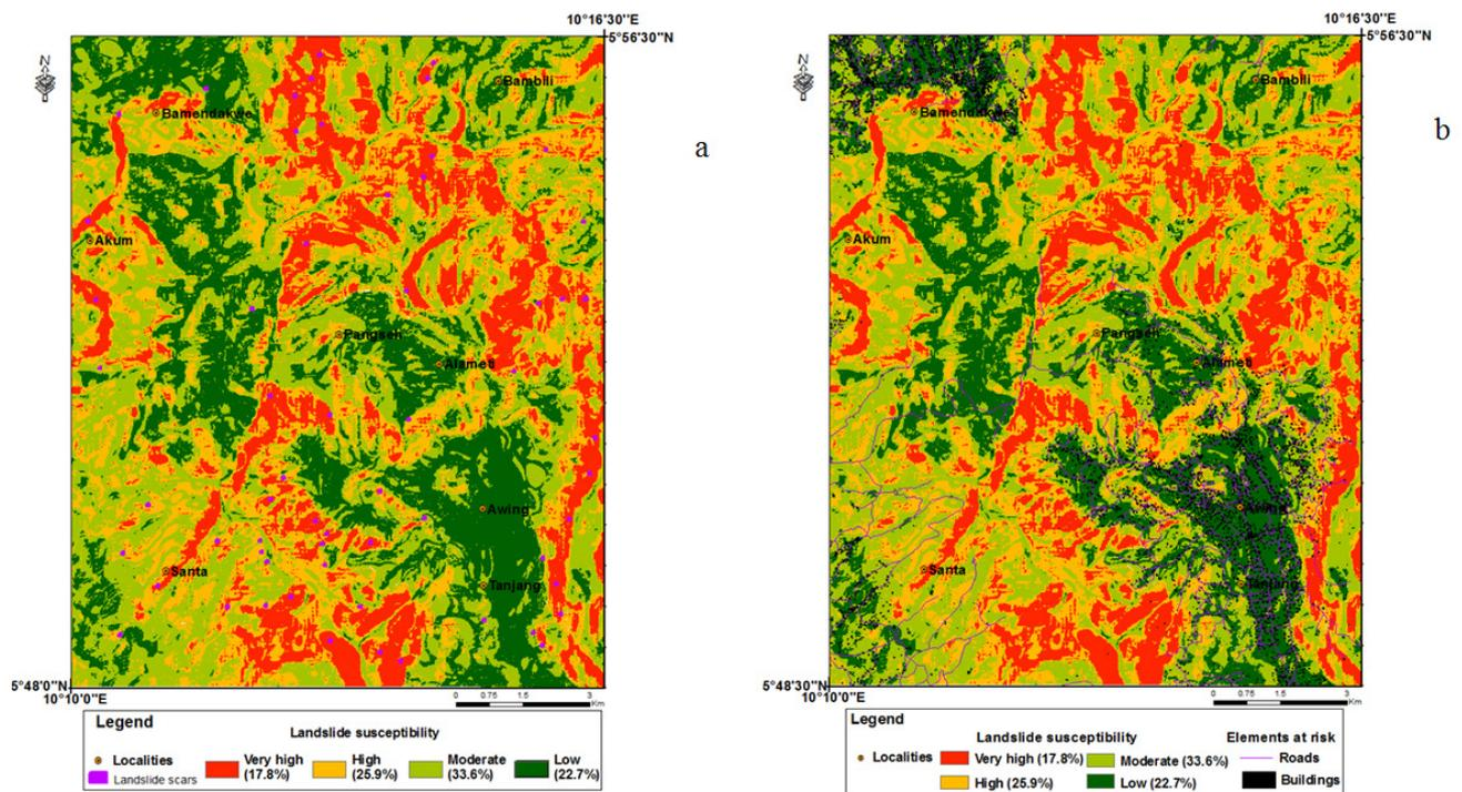
**Figure 4.** (a) Classified landslide susceptibility map of the Bamenda Mountain (landslide scars have been magnified) (b) Landslide risk map of the Bamenda Mountain
