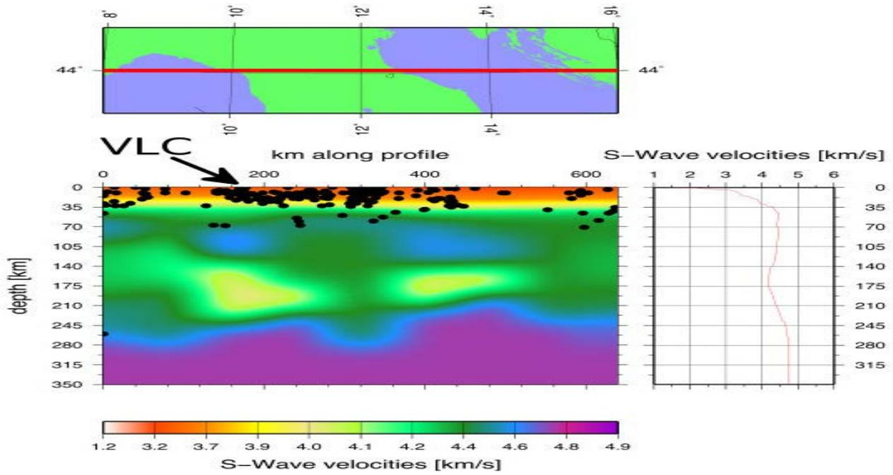
Figure 7. Shear wave velocity cross-section of the study area with distribution of earthquake hypocenters (black dots) with depth
