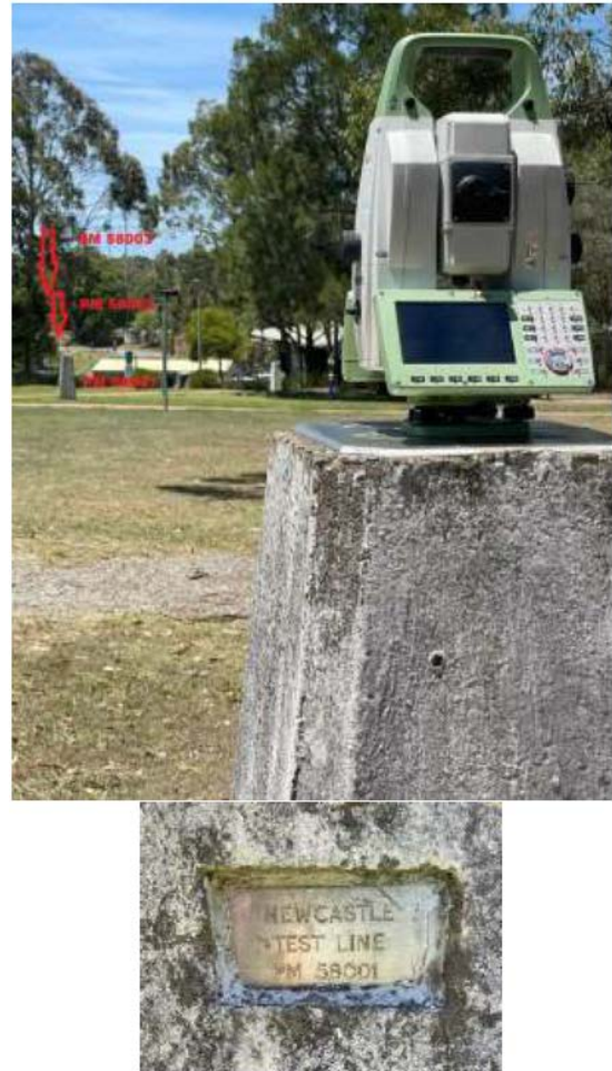
Figure 7. above: Four known benchmarks shown; MS60 was levelled on the PM 58000 pillar, below: The photo taken from the pillar PM 58001 (as Newcastle Test Baseline)
