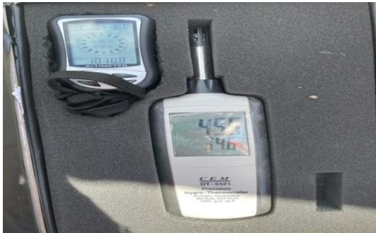
Figure 8. Thermo-meters and barometers used to record the temperature and pressure during measurements
