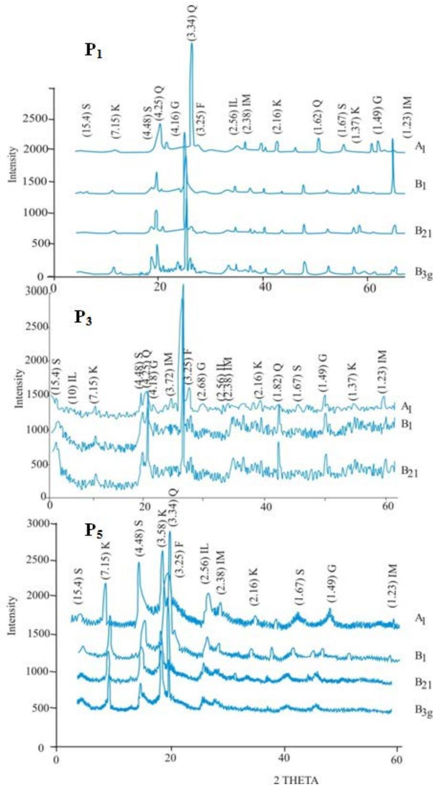
**Figure 3.** X-ray diffraction patterns of Vertisol horizons from Garoua (P<sub>1</sub>), Bounguel (P<sub>3</sub>) and Karewa (P<sub>5</sub>). (S = smectite; = Kaolinite; IL = Illite; IM = Ilmenite; F = Feldspar; G = Goethite; Q = Quartz)
