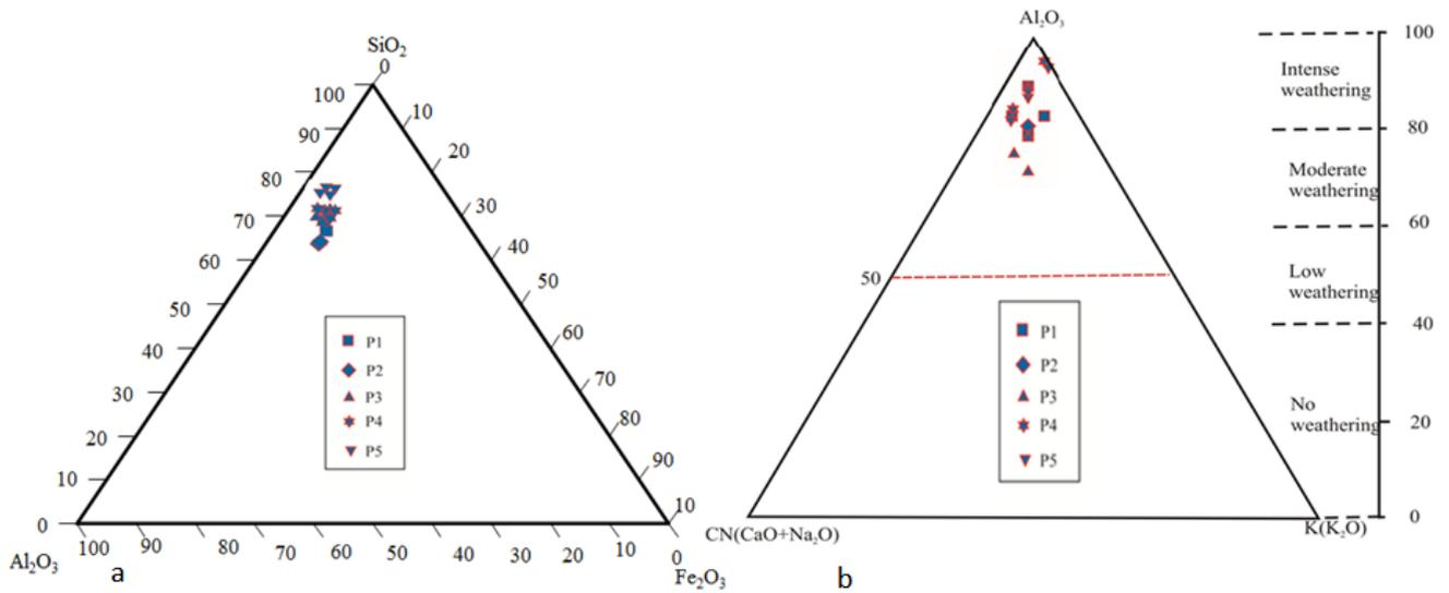
**Figure 5.** Triangular diagrams of geochemical data. (a) SiO<sub>2</sub>-Al<sub>2</sub>O<sub>3</sub>-Fe<sub>2</sub>O<sub>3</sub> triangular plot of the Vertisols; (b) Al<sub>2</sub>O<sub>3</sub>-(CaO\*+Na<sub>2</sub>O)-K<sub>2</sub>O (A-CN-K) triangular diagram illustrating the degree of chemical weathering in reference to [29]
