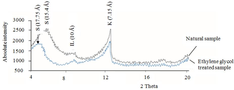
**Figure 4.** X-ray diffraction of the A1 horizon (0-30 cm) from the Benue Basin Vertisols after treatment with ethylene glycol (S= smectite; K= kaolinite; I = Illite)
