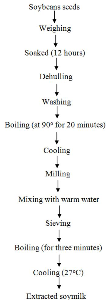
Figure 2. Flow diagram for extraction of Soymilk
