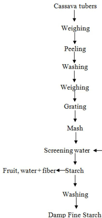
Figure 1. Flow diagram for starch extraction
