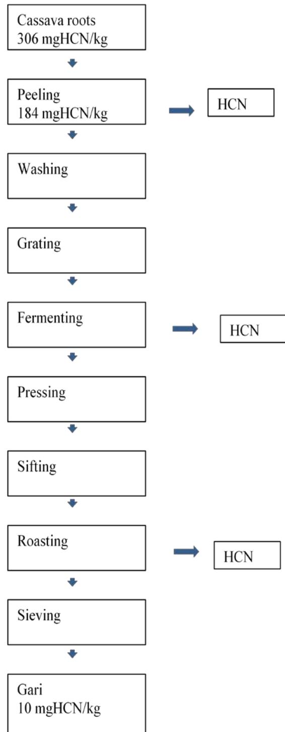
**Figure 1.** Process flow chart for gari production showing points of cyanide removal (HCN values cited from [78])
