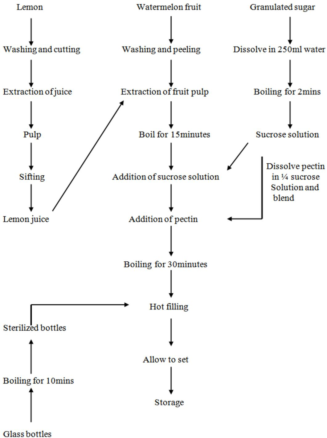
Figure 1. Process flow chart for watermelon jam
