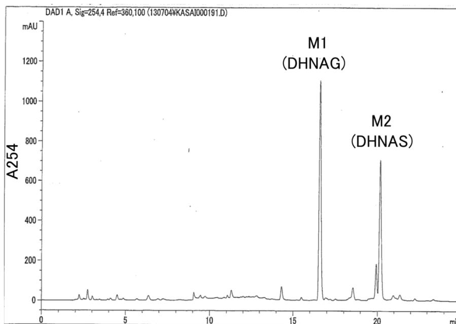
Figure 2. Analysis of DHNA metabolites in mouse urine. After DHNA administration to mice, a portion of the 24 h urine sample was analyzed by HPLC
