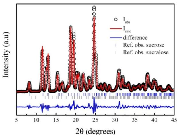
Figure 1. Rietveld refining of sugar fit, obtained from supplier
