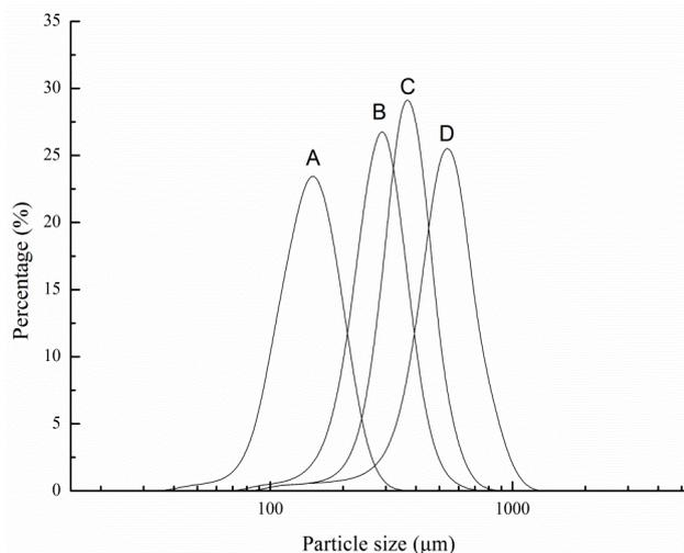
**Figure 1.** The particle size distribution curves of wheat bran and wheat flour (A: wheat bran passing through 100 meshes; B: wheat bran passing through 80 meshes; C: wheat bran passing through 60 meshes; D: wheat bran passing through 40 meshes.)
