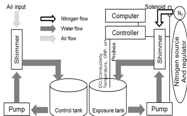
Figure 1. Schematic diagram of the hypoxia chamber
