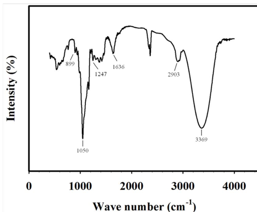
**Figure 3.** Fourier transform infrared spectroscopy of mixed  $< 3\text{ kDa}$   $\beta$ -1,3-xylooligosaccharide
