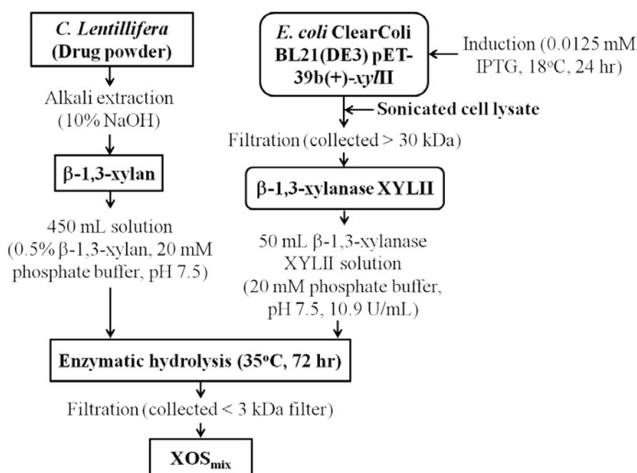
Figure 1. Schematic diagram of the preparation of  $\text{XOS}_{\text{mix}}$ .
