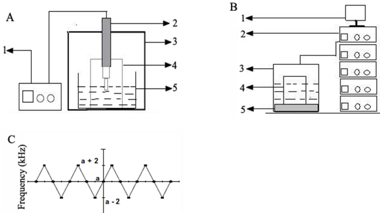
**Figure 1.** (A–C) (A) Schematic diagram of probe ultrasound pretreatment 1. Ultrasonic controller. 2. Probe ultrasound. 3. Acoustic chamber. 4. Sample pretreatment beaker. 5. Thermostatic water bath. (B) Schematic diagram of flat plate ultrasound pretreatment. 1. Computer. 2. Frequency controller. 3. Ultrasonic tank. 4. Sample pretreatment beaker. 5. Flat plate ultrasound. (C) Frequency variation curve of ultrasound for sweep model
