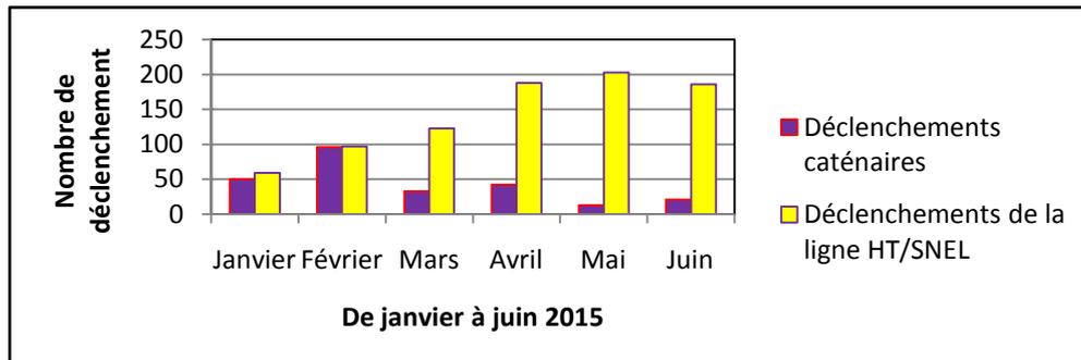
Figure 8. Statistics of tripping operations in all substations SNCC from January to June 2015
