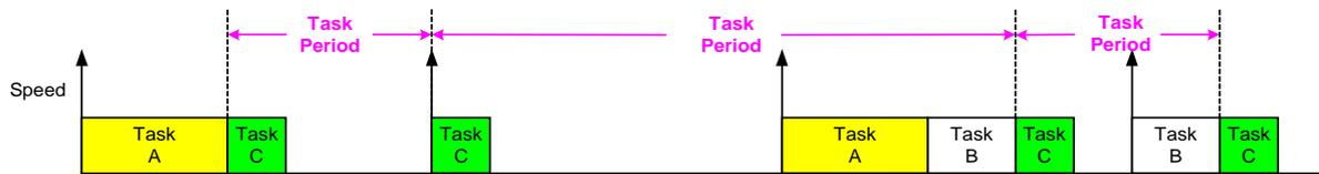
Figure 2. Release jitter caused by task placement in TTC schedulers
