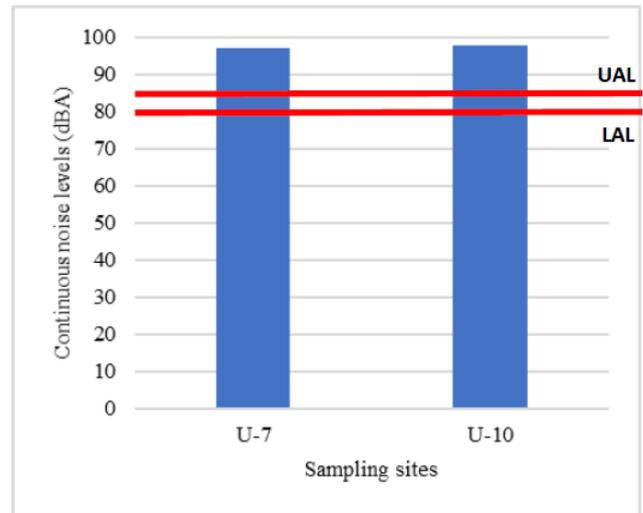
**Figure 5.** Continuous noise levels from automotive workshop sources at different sampling sites
