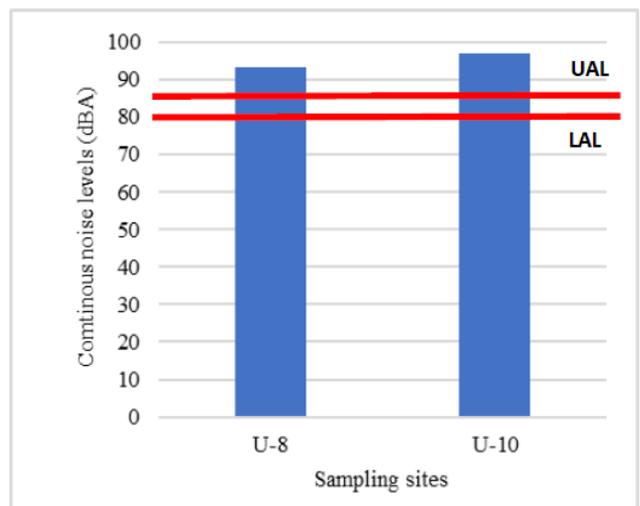
**Figure 3.** Continuous noise levels for heavy construction plant equipment at different sampling sites
