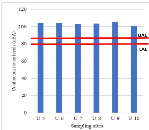
**Figure 8.** Continuous noise levels from welding workshop sources at different sampling sites
