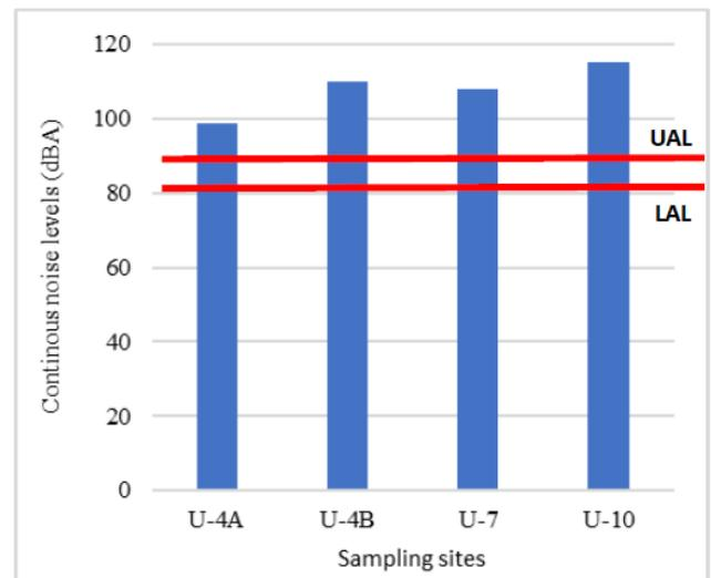
**Figure 9.** Continuous noise levels for other workshop activities at different sampling sites. U-4A, mineral processing lab; U-4B, foundry workshop; U-7, aerospace engineering lab
