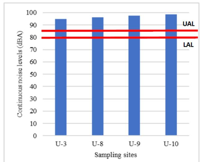
**Figure 6.** Continuous noise from carpentry workshop sources at different sampling sites
