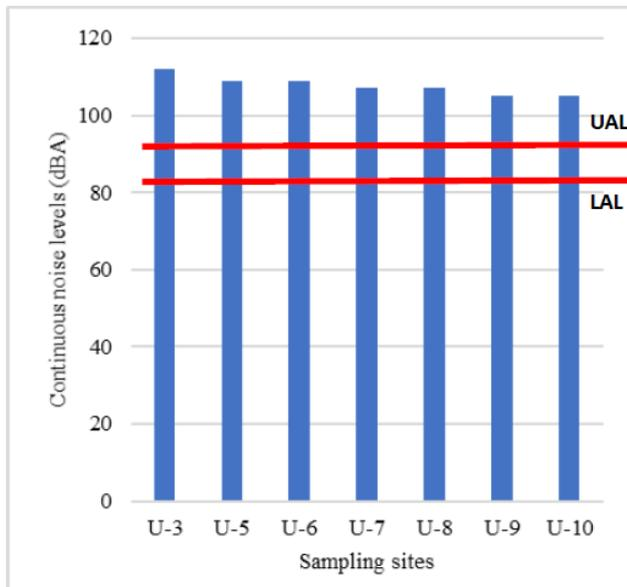
**Figure 7.** Continuous noise levels from thermodynamics lab sources at different sampling sites
