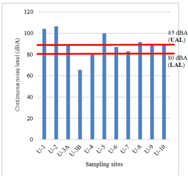
**Figure 1.** Continuous noise levels for machine workshops at different sampling sites. UAL, upper action limit; LAL, lower action limit [29]
