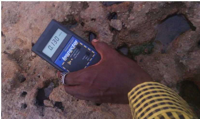
Plate 1. Radiation detector equipment put to use on-site
