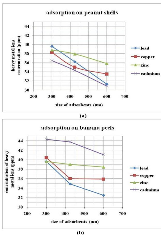
Figure 2. (a) Adsorption of metal ions on peanut shells; (b) Adsorption of metal ions on banana peels
