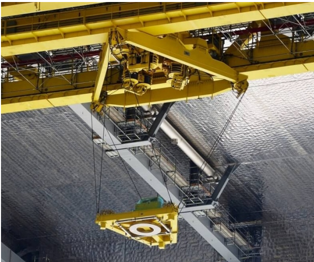
Figure 2. The NIST RoboCrane (six-cable-suspended robot)
