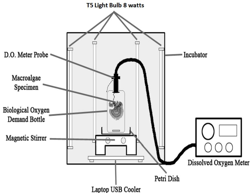
Figure 1. Schematic diagram of the incubating chamber
