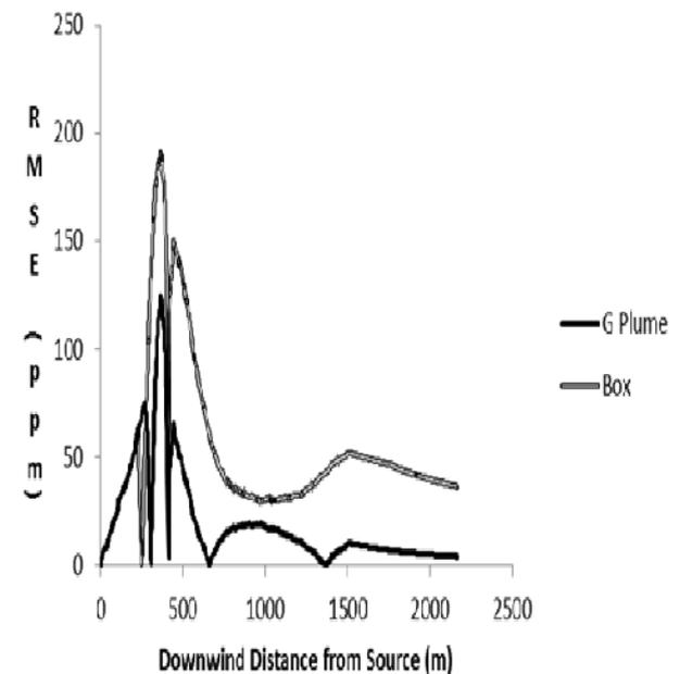
Figure 6b. Calculated RMSE profile for the NO<sub>2</sub> concentration at the Baldwin location
