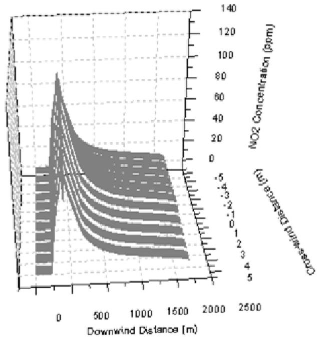
Figure 4e. NO<sub>2</sub> concentration profile for the Baldwin location calculated by the Box Model
