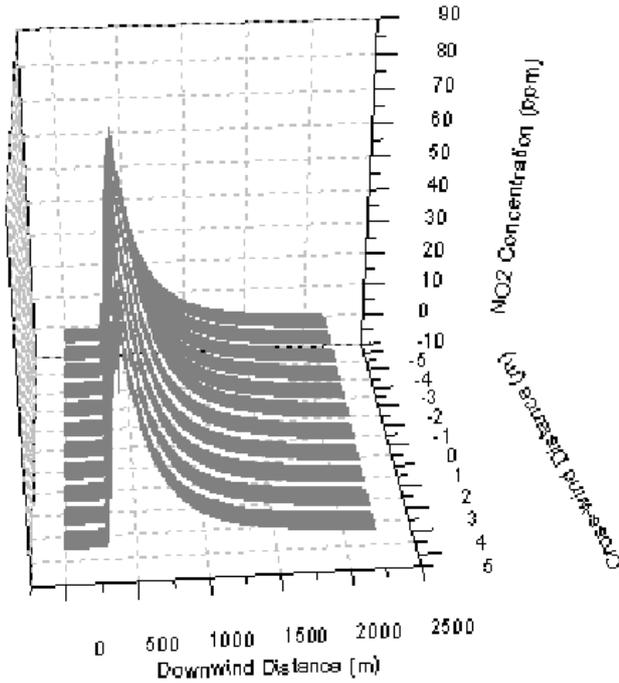
Figure 4c. NO<sub>2</sub> concentration profile for the Baldwin location calculated by the Variable K Model
