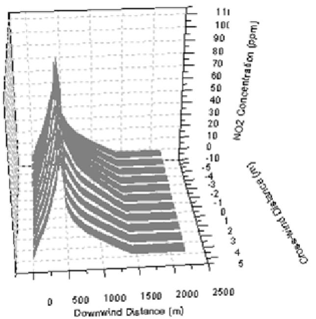
Figure 4b. NO<sub>2</sub> concentration profile for the Baldwin location calculated by the Gaussian Plume Model
