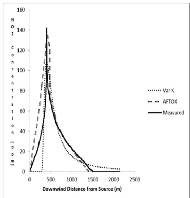
Figure 5a. Calculated NO<sub>2</sub> concentration profile at the Baldwin location
