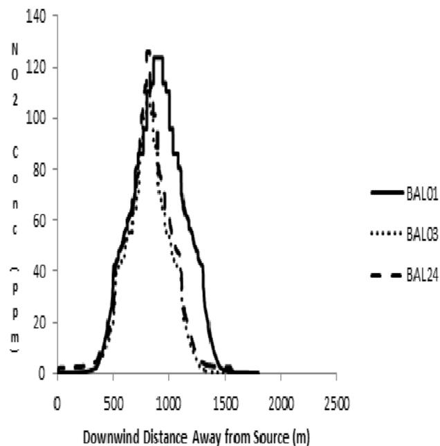
Figure 2. NO<sub>2</sub> concentration profile for the Baldwin location
