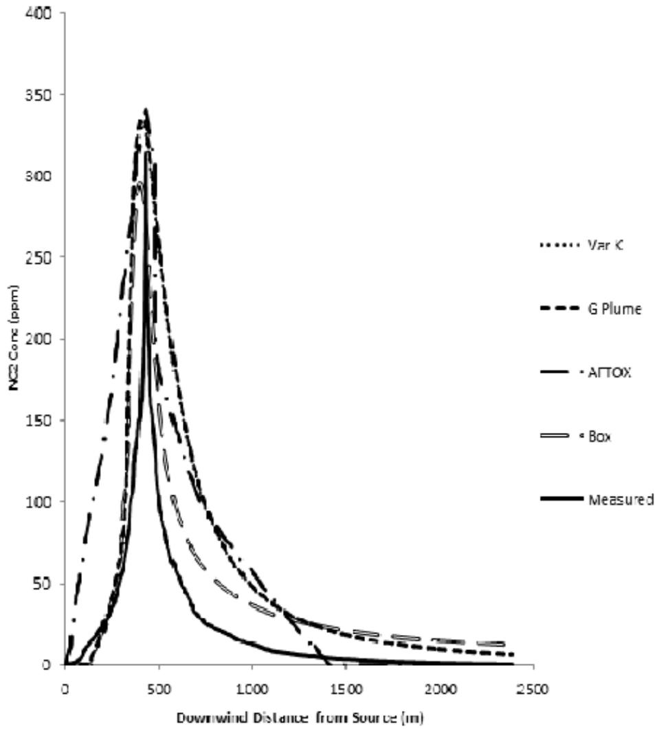
Figure 3. Calibrated NO<sub>2</sub> concentration profile for the Westvaco location
