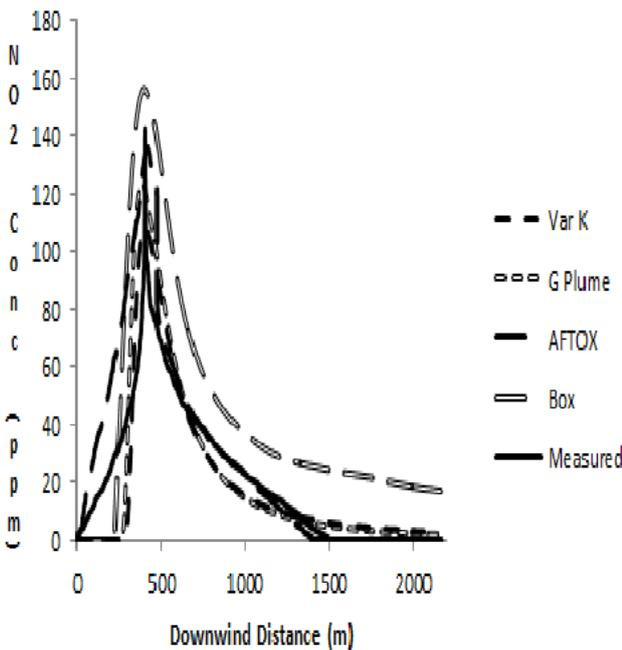
Figure 5c. Calculated NO<sub>2</sub> concentration profile at the Baldwin location
