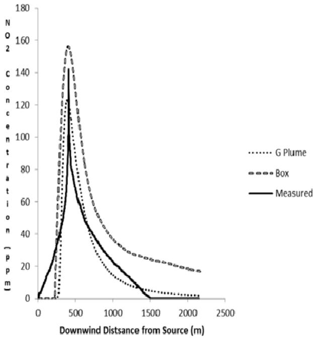
Figure 5b. Calculated NO<sub>2</sub> concentration profile at the Baldwin location
