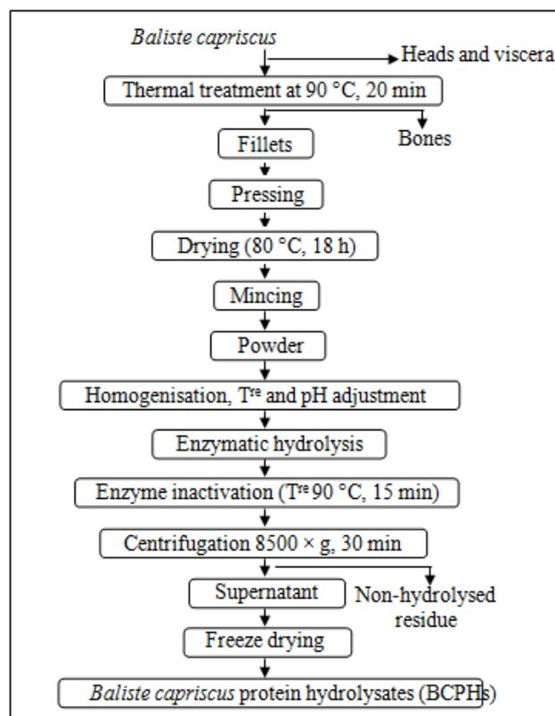
Figure 1. Flow sheet for preparation of BPHs
