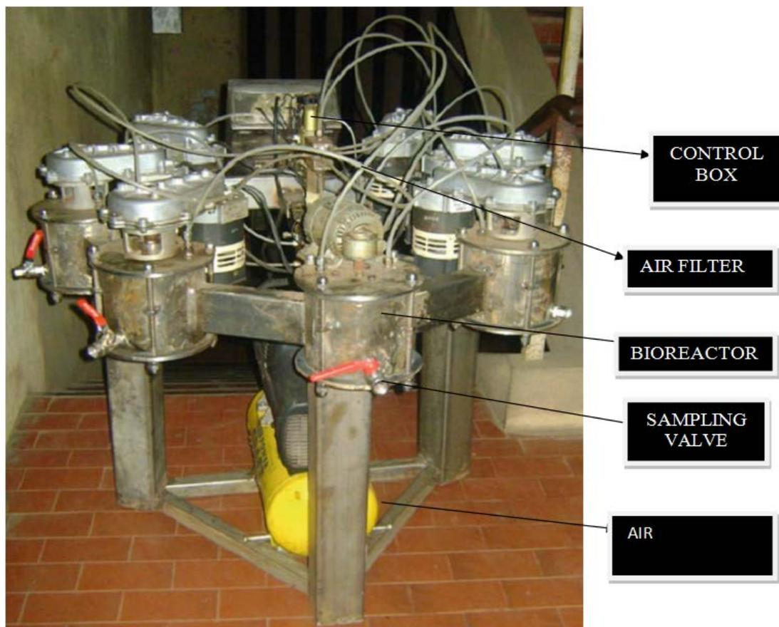
**Figure 1a.** The seven 2.5 L bioreactors (Source: Chikere *et al.* 2012)
