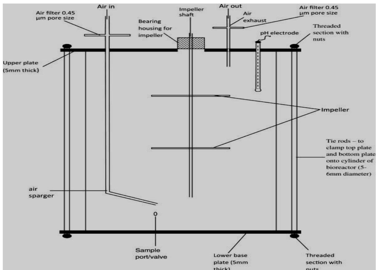
Figure 1b. The interior design of the 2.5 l bioreactors (Source: Chikere *et al.* 2012)
