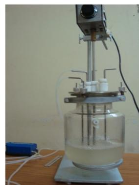
Figure 1. Bioreactor
