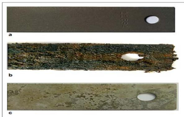
**Figure 2.** Mild steel coupon: a – new, unexposed coupon, b – coupon retrieved from the water-logged soil site, c – coupon after cleaning
