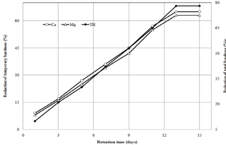
Figure 3. Effect of retention time on reduction of total hardness and temporary hardness
