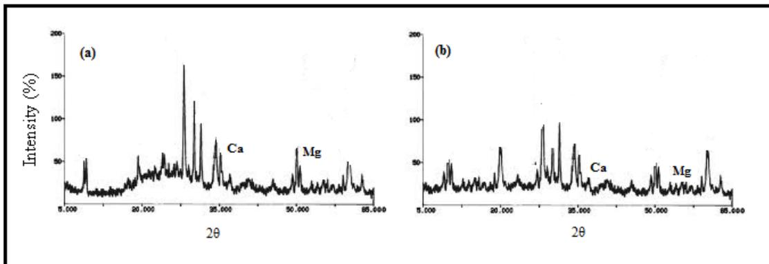
Figure 5. X-ray diffraction of hardness reduction studied (a) before treatment (b) after treatment
