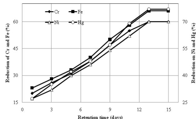
Figure 2. Effect of retention time on heavy metal reduction
