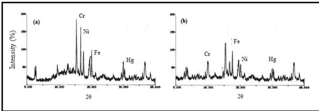
Figure 4. X-ray diffraction of heavy metal reduction studied (a) before treatment (b) after treatment
