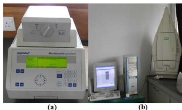
Figure 2. (a) Eppendorf- Mastercycler gradient, thermal cycler, (b) BIORAD gel documentation system
