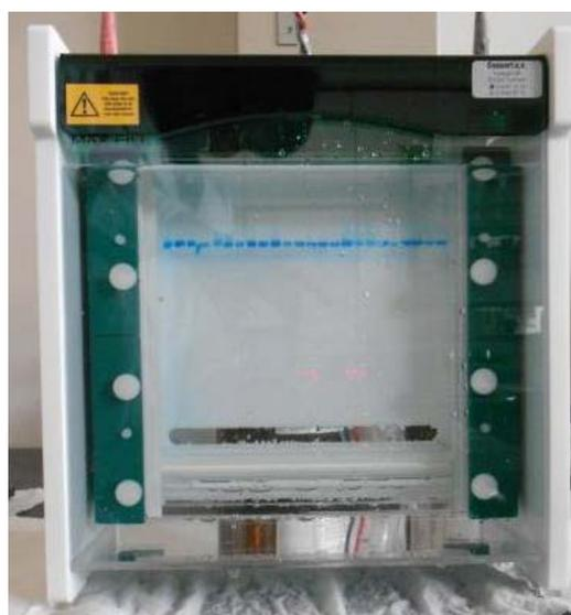
**Figure 3.** Polyacrylamide gel electrophoresis apparatus
