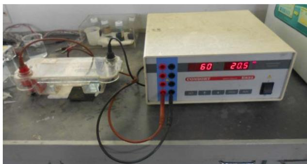
Figure 1. Agarose gel electrophoresis apparatus
