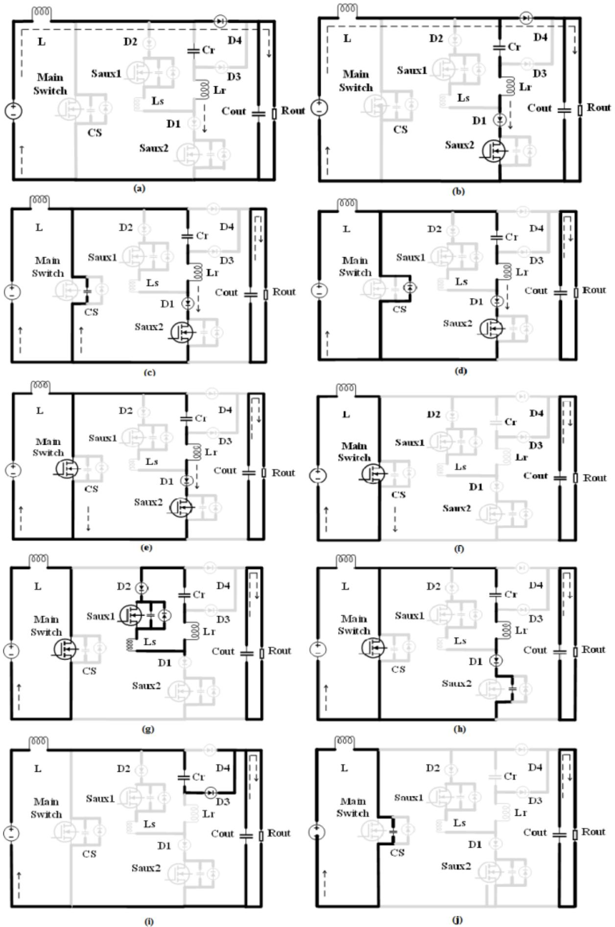
Figure 9. 10 State's proposed soft switch inverter
