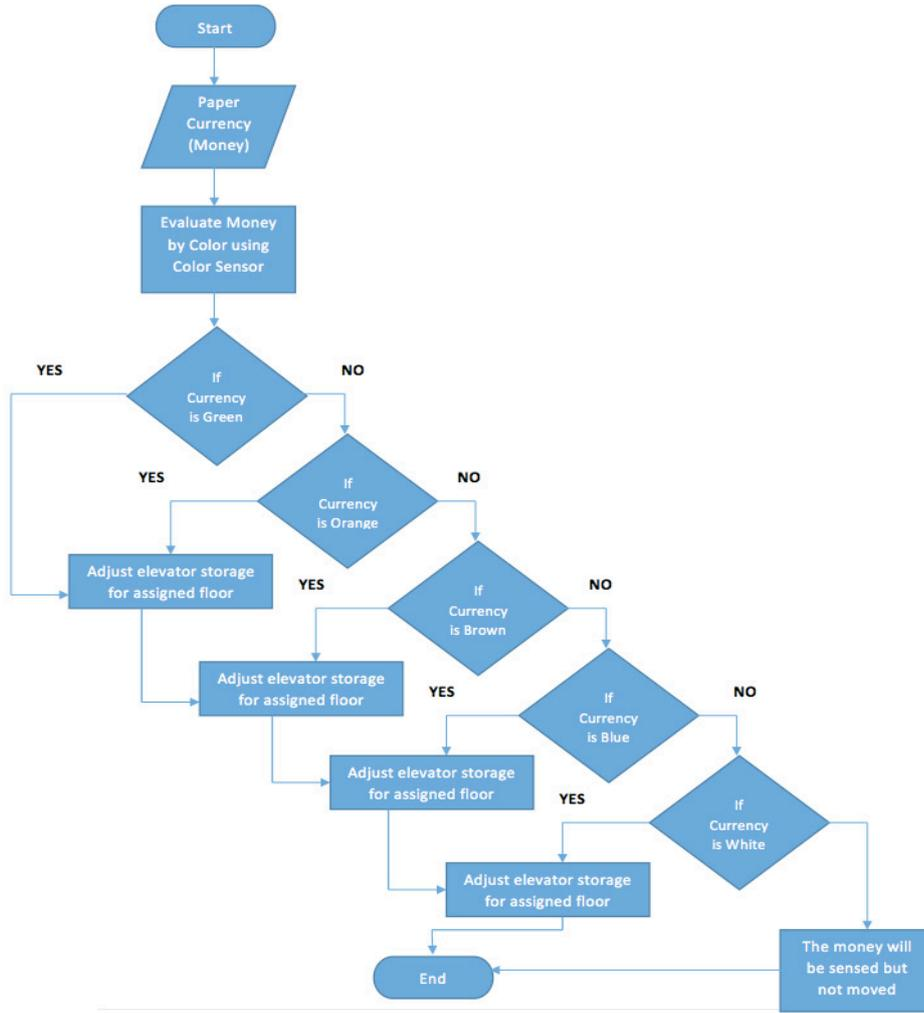
Figure 6. System Flowchart of the Design
