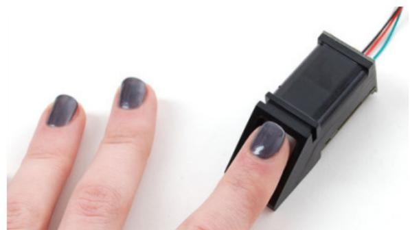
Figure 5. Fingerprint Scanner
