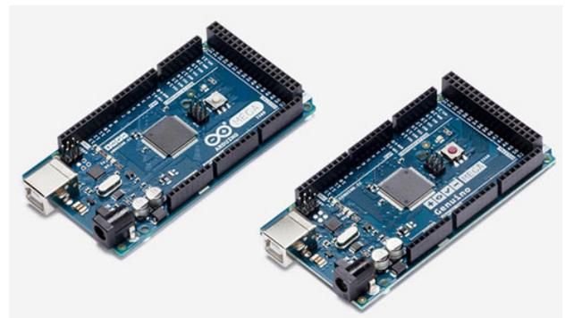
Figure 1. Arduino Mega 2560 Controller
