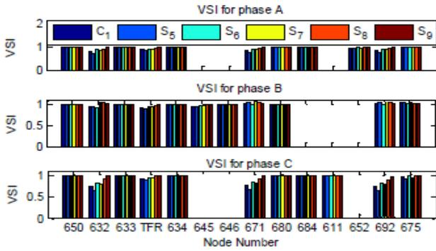
Figure 18. VSI for Category B V2G Interconnection of IEEE 13 Test Feeder
