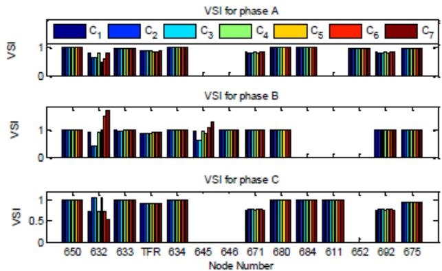
Figure 6. VSI for IEEE 13 Node Test Feeder for V2G Interconnection at Phase B
