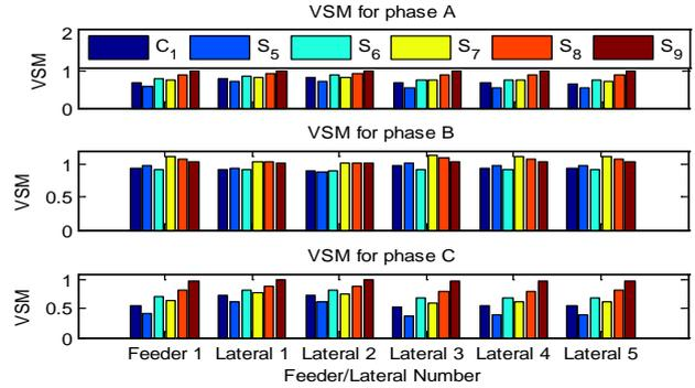
Figure 19. 3-Phase VSM for Category B V2G Interconnection of IEEE 13 Feeder
