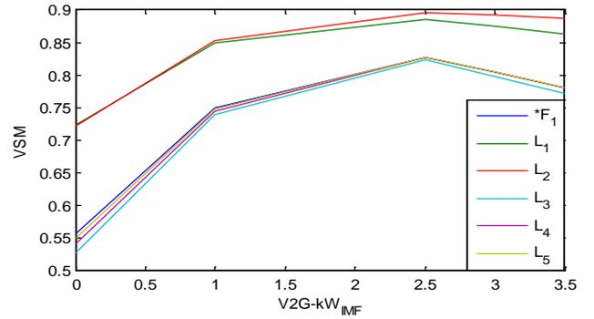
**Figure 24.** Variation of VSM of all laterals of 13-Node system with  $kW_{IMF}$
