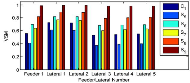
Figure 20. System VSM for Category B V2G Interconnection of IEEE 13 Feeder
