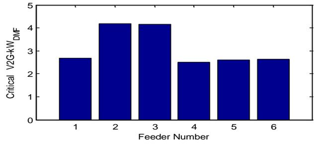
**Figure 23.**  $V2G-kW_{DMF}$  required to initiate voltage collapse for IEEE 13 Feeder.
