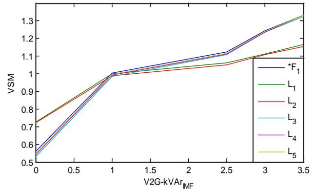
**Figure 25.** Variation of VSM of all laterals of 13-Node system with  $kvar_{IMF}$
