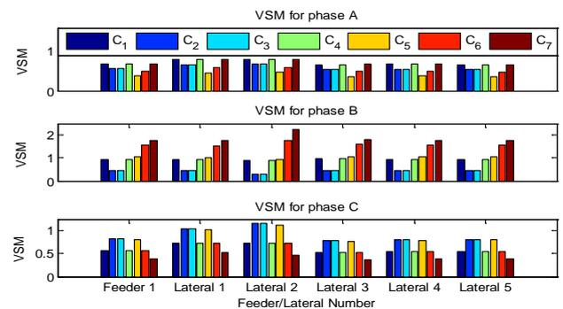
Figure 7. VSM for IEEE 13 Test Feeder for V2G Interconnection at Phase B
