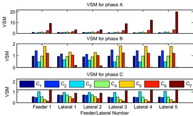
Figure 3. VSM for IEEE 13 Test Feeder for V2G Interconnection at Phase A
