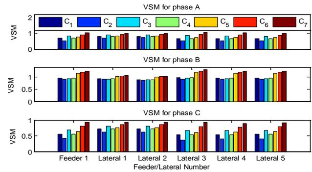
Figure 15. VSM of Laterals for 3-phase V2G Interconnection of IEEE 13 Feeder
