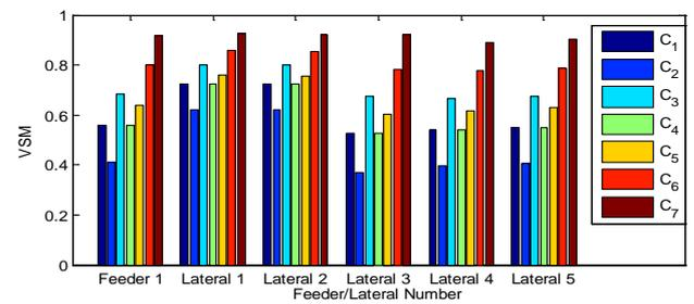
Figure 16. Lateral VSM for 3-phase V2G Interconnection of IEEE 13 Feeder
