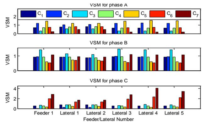
**Figure 11.** 3-phase VSM for V2G Interconnection at Phase C of IEEE 13 Feeder
