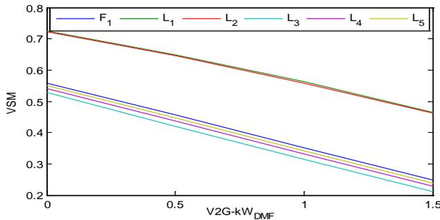
**Figure 22.** Variation of VSM of all laterals of 13-Node system with  $kW_{DMF}$
