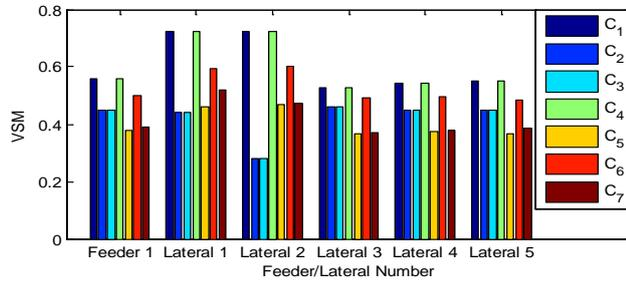
**Figure 8.** System VSM for V2G Interconnection at Phase B of IEEE 13 System
