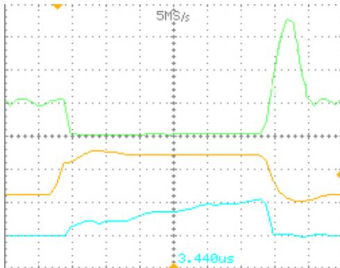
Figure 8. Drain-source voltage and current (dashed) waveforms of main switch S (vertical scale 25V/div or 2.5A/div, time scale 1μs/div)
