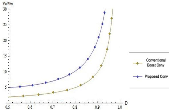
Figure 4. proposed converter gain compared with conventional boost converter versus duty cycle
