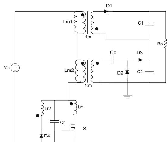
Figure 1. The proposed step-up converter with auxiliary circuit
