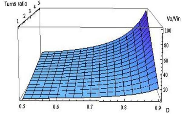
Figure 5. 3D plot of gain versus turns ratio and duty cycle
