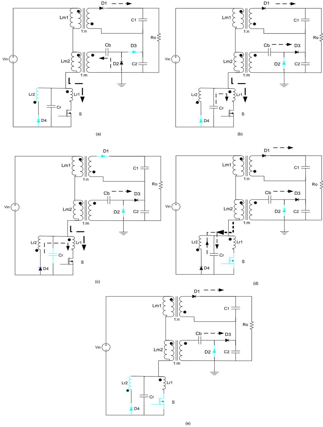
**Figure 3.** Equivalent circuits for each operating interval of the proposed converter: (a): $t_0-t_1$ , (b): $t_1-t_2$ , (c): $t_2-t_3$ , (d): $t_3-t_4$ , (e): $t_4-t_0$ , (The gray colored elements do not conduct current)
