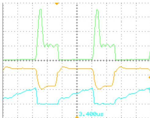
Figure 9. Drain-source voltage and current (dashed) waveforms of main switch S (vertical scale 25V/div or 2.5A/div, time scale 1μs/div)
