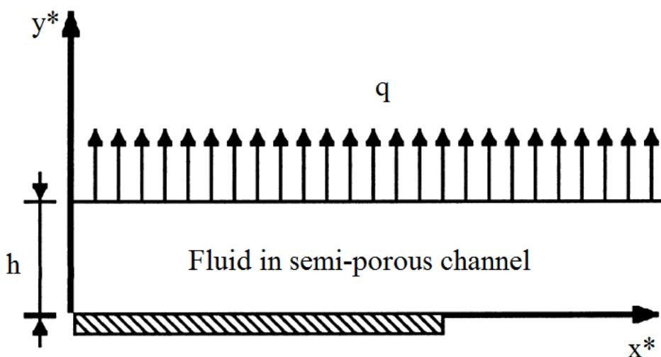
Figure 1. Schematic of the problem (fluid in a porous media between parallel plates and magnetic field)
