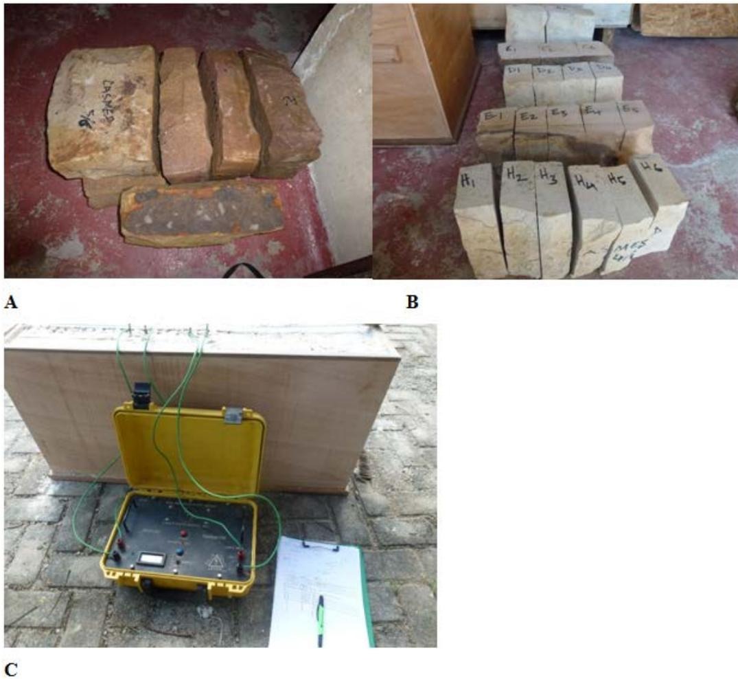
**Figure 3.** Experimental system and procedure used for studying Effect of Fracture Intensity and Aperture Size. (A) Rock blocks (B) Series of rock blocks use as fracture samples, (C) Experimental setup (Dipole-Dipole configuration)
