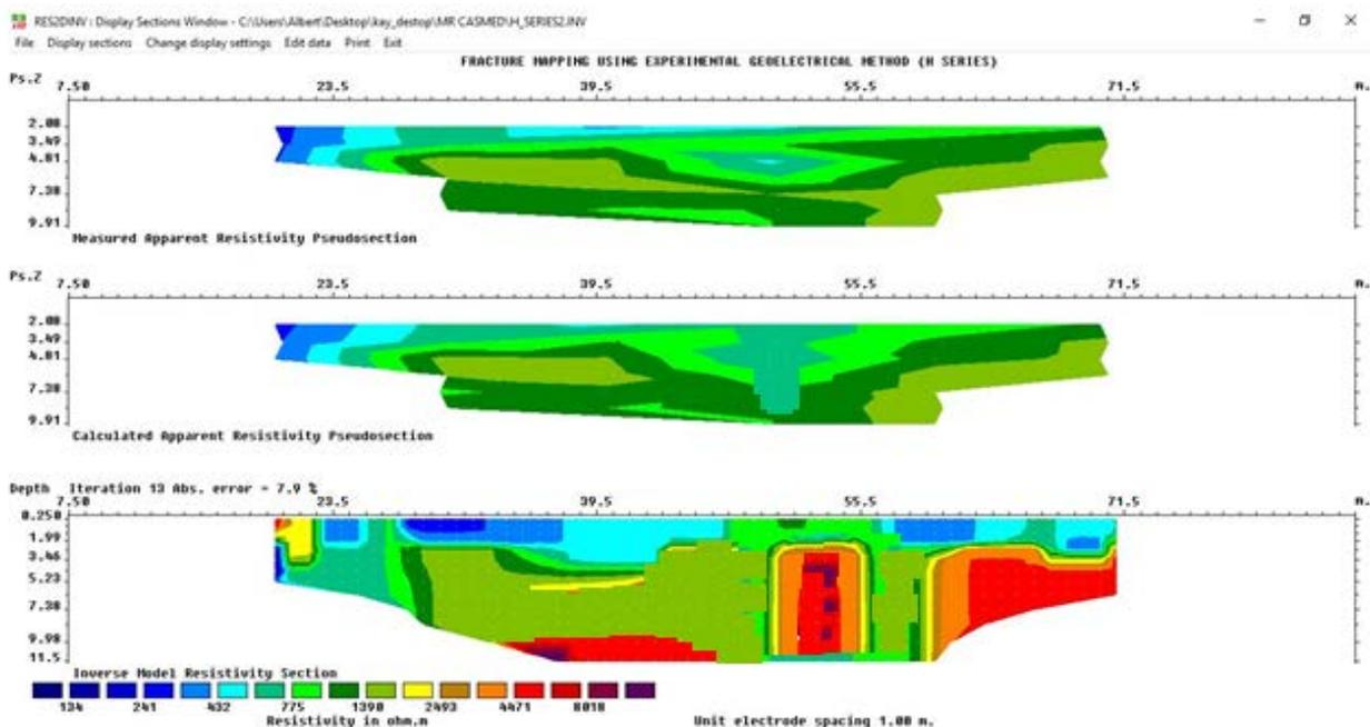
Figure 7. Electrical image across the vertical fracture with aperture of 6 mm between the comparatively lower resistivity quartzite rock block
