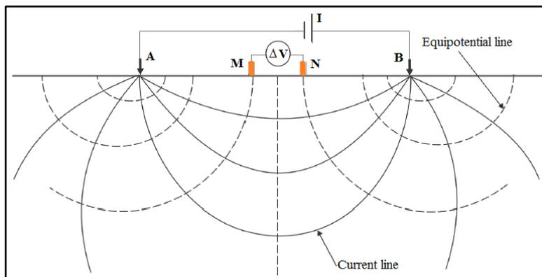
**Figure 2.** Field Acquisition of Resistivity data (Modified from [10])
