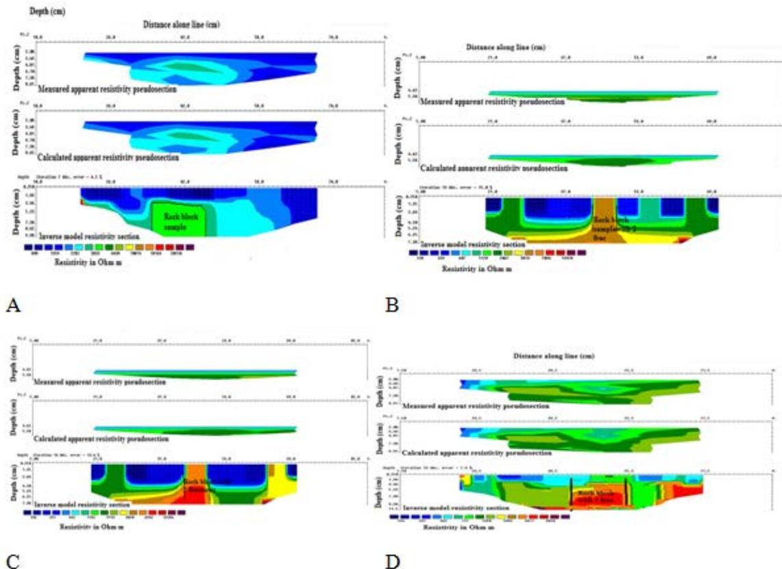
**Figure 5.** Samples of 2D Apparent Resistivity Pseudosections of the Laboratory Experiments. (A) Sample block with 2 Fractures, (B) Block with 2 Fractures, (C) Block with 4 Fractures, (D) Block with 5 Fractures
