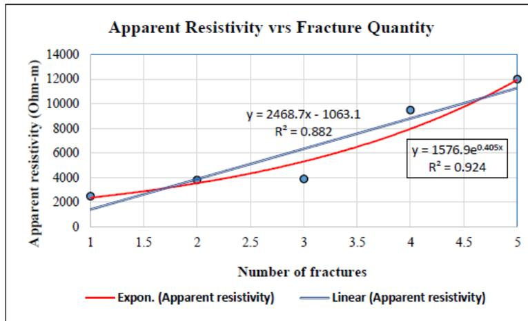
Figure 6. Apparent resistivity versus fracture quantity
