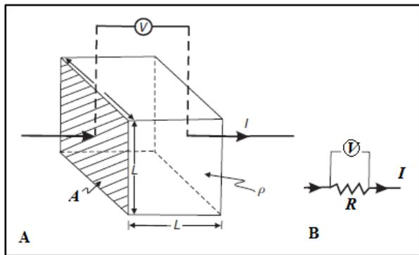
**Figure 1.** Parameters used in defining resistivity. (A) Definition of resistivity across a block of side length  $L$  with an applied current  $I$  and potential drop between opposite faces of  $V$ . (B) Electrical circuit equivalent,  $R$  is a resistor (Modified after Reynold, [2])
