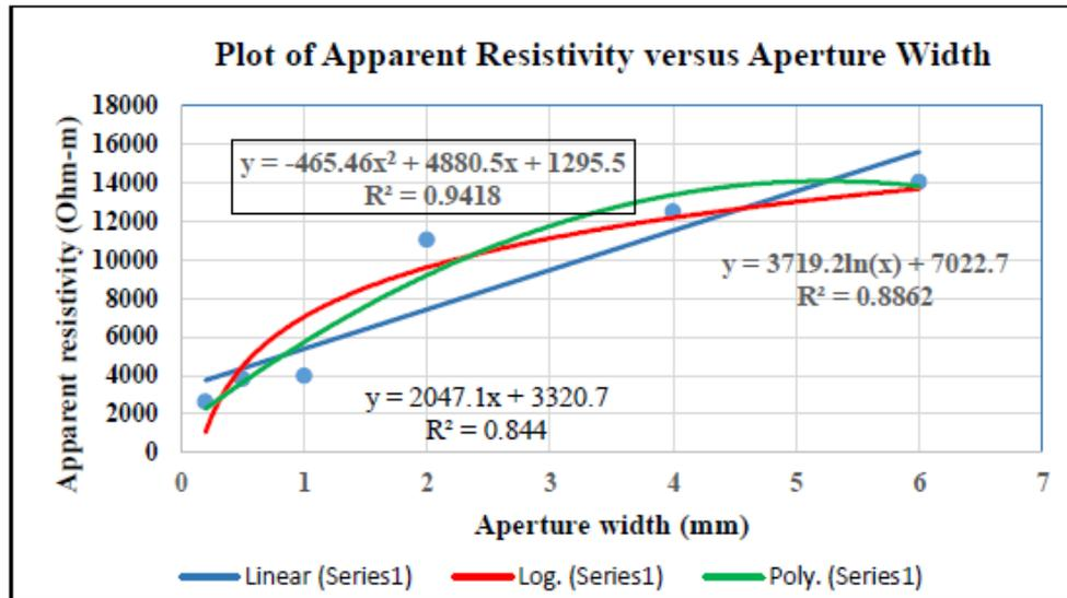
Figure 8. Apparent resistivity versus Aperture Width
