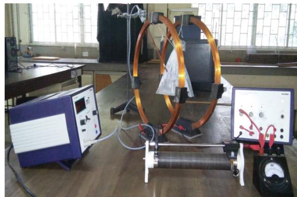
Plate 1. Experimental setup for water samples magnetic B-field application
