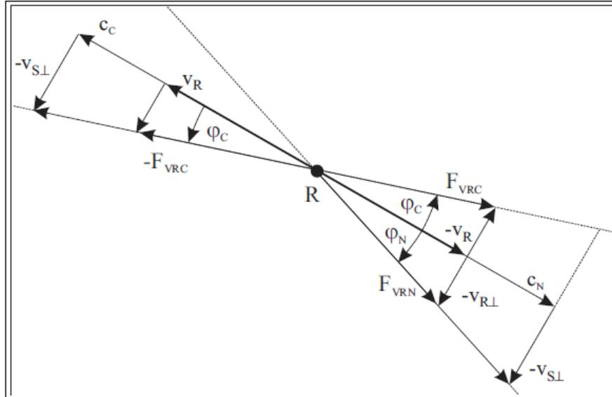
Figure 3. Forces on R with  $v_{S\perp}$
