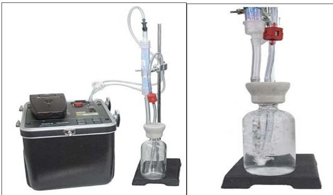
Figure 2. Measurement apparatus RAD
