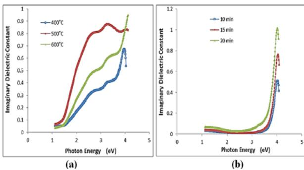
**Figure 11.** Imaginary dielectric constant as a function of photon energy of CuO thin films:(a) furnace annealing (b) laser annealing
