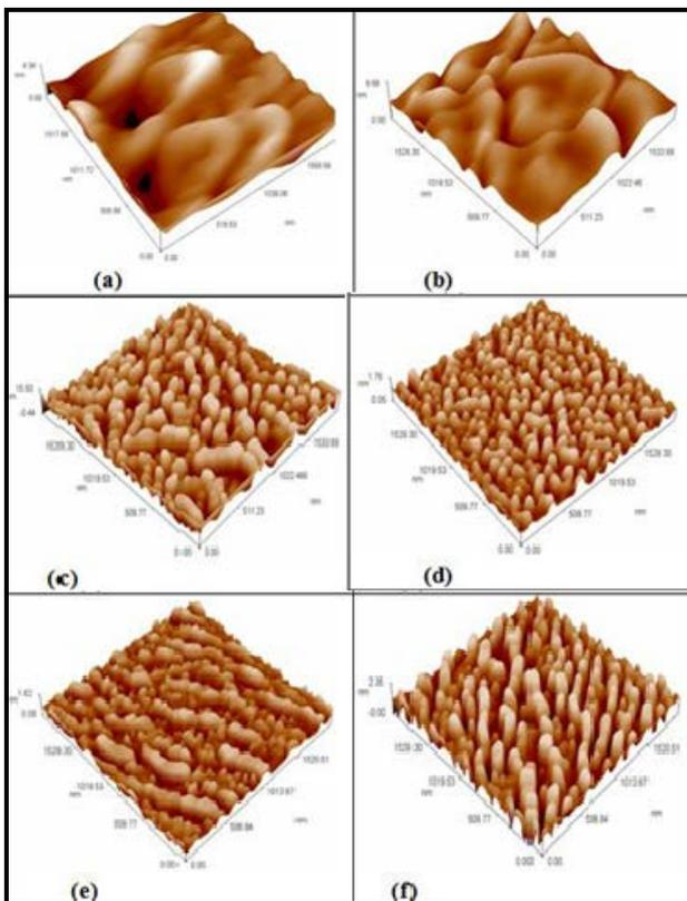
**Figure 2.** AFM image of copper oxide thin films which annealed: (a) by oven at (400 °C), (b) by oven at (500 °C), (c) by oven at (600 °C), (d) by laser for (10 min), (e) by laser for (15 min), (f) by laser for (20 min)
