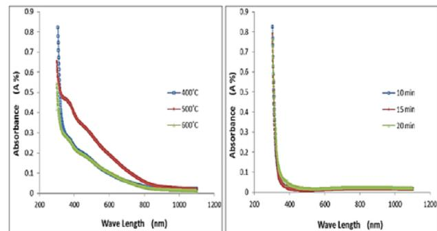
**Figure 4.** Absorbance spectrum of CuO thin films: (a) furnace annealing (b) laser annealing
