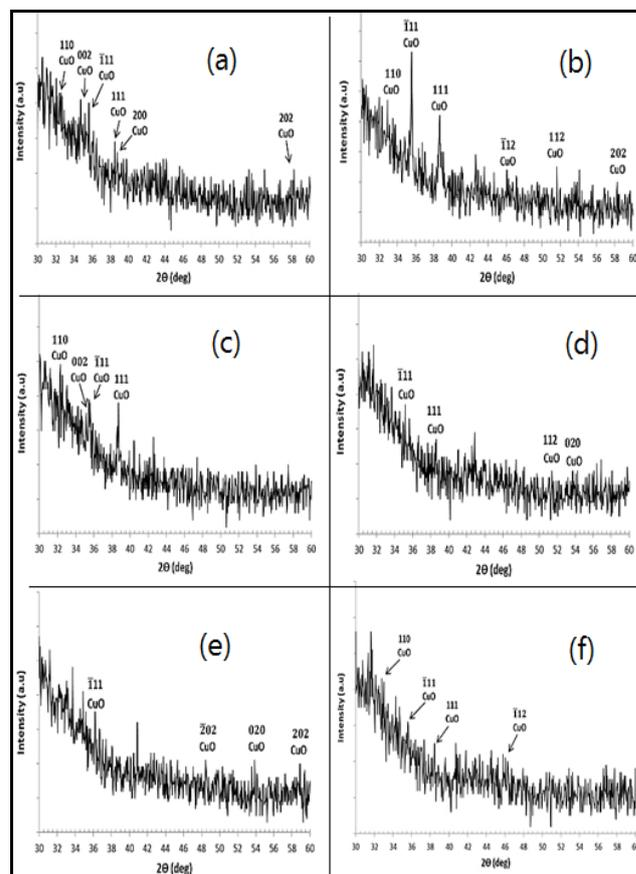
**Figure 1.** X-ray diffraction scheme of the copper oxide thin films which annealed:(a) by oven at ( $400^\circ\text{C}$ ), (b) by oven at ( $500^\circ\text{C}$ ), (c) by oven at ( $600^\circ\text{C}$ ), (d) by laser for (10 min), (e) by laser for (15 min), (f) by laser for (20 min)
