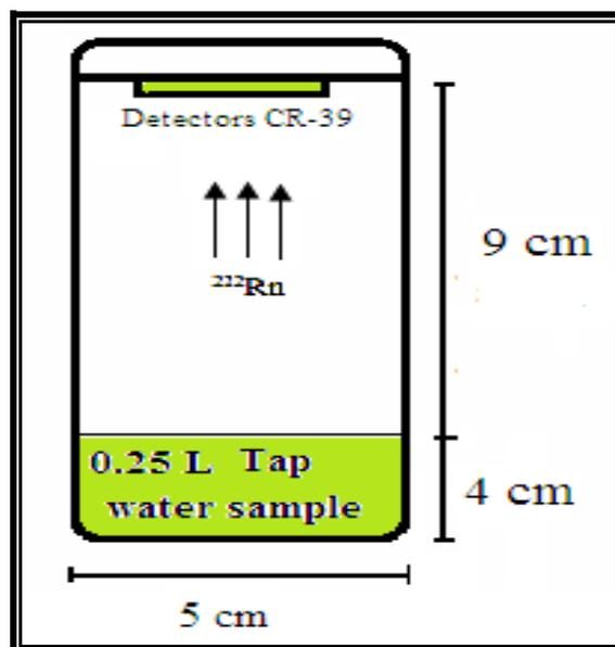
**Figure 2.** sealed-cup technique used for water samples
