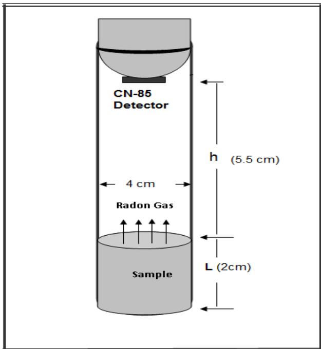
Figure 2. Experimental setup for measurements of radium concentration and radon exhalation rates in soil samples
