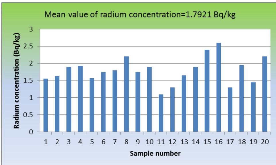
Figure 5. Radium concentration of the soil samples from the Kerbala governorate
