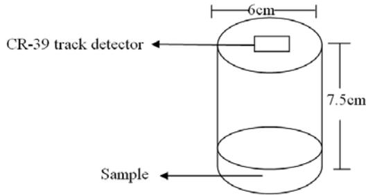
Figure 1. Sealed Can Technique
