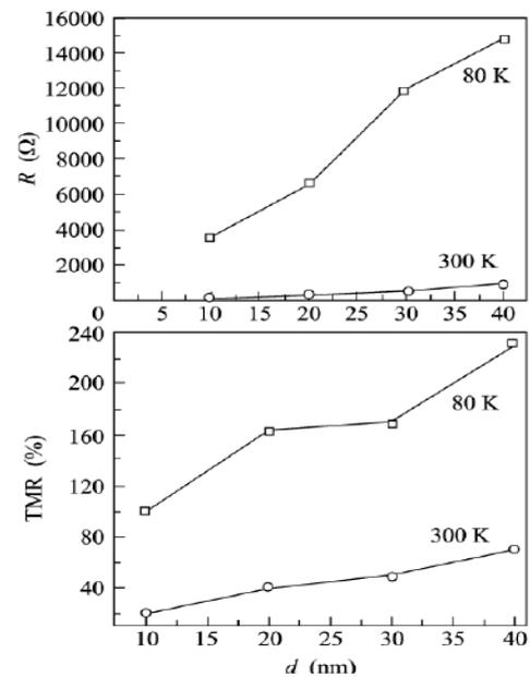
**Figure 1.** (Upper panel) Tunneling resistance  $R$  and (lower panel) magnetoresistance TMR of the  $\text{SiO}_2/\text{Tb}_{19}\text{Co}_5\text{Fe}_{76}/\text{Pr}_6\text{O}_{11}/\text{Tb}_{22}\text{Co}_5\text{Fe}_{73}/\text{SiO}_2$  film structure versus the thickness of the  $\text{Pr}_6\text{O}_{11}$  barrier layer
