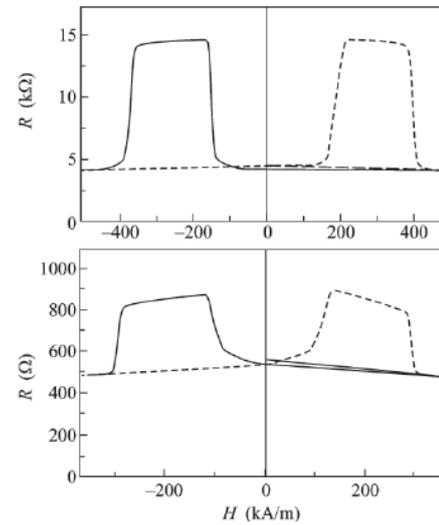
**Figure 4.** Resistance of the  $\text{SiO}_2/\text{Tb}_{19}\text{Co}_5\text{Fe}_{76}/\text{Pr}_6\text{O}_{11}/\text{Tb}_{22}\text{Co}_5\text{Fe}_{73}/\text{SiO}_2$  tunneling contact versus the applied magnetic field at  $T = 80$  K (upper panel) and  $T = 300$  K (lower panel)
