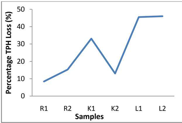
Figure 20. Percentage Total Petroleum Hydrocarbon Loss of Samples
