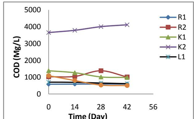
Figure 8. Variation in Chemical Oxygen Demand Level of the Samples during the Degradation
