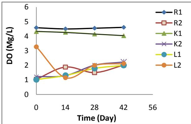
Figure 2. Variation in Dissolved Oxygen Level of the Samples during the Degradation
