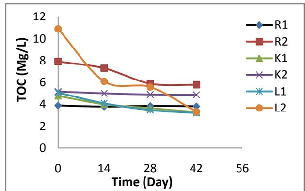
Figure 7. Variation in Total Organic Carbon Level of the Samples during the Degradation
