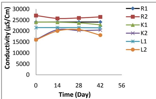
Figure 3. Variation in Conductivity Level of the Samples during the Degradation
