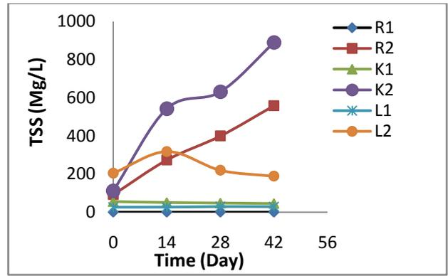
Figure 5. Variation in Total Suspended Solids Level of the Samples during the Degradation
