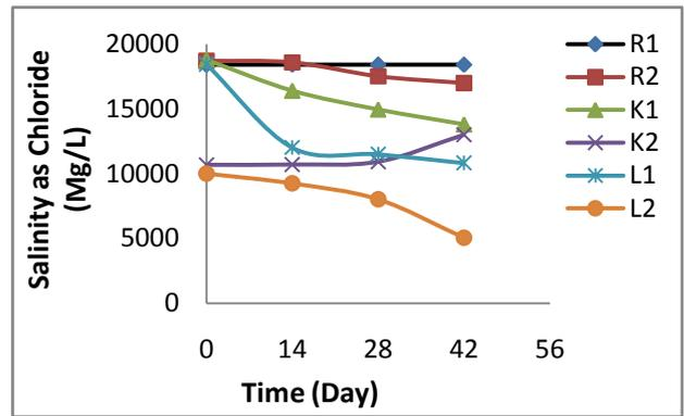
Figure 6. Variation in Salinity Level of the Samples during the Degradation
