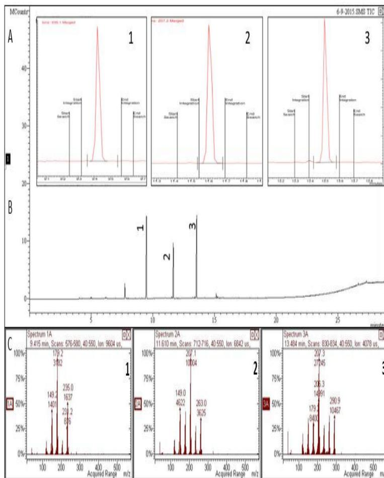
**Figure 3.** Identification of MBT (peak 1), DBT (peak 2) and TBT (peak 3) of known samples (B) chromatographic separation and (C) mass spectrum of each compound). Showing unique fragmentation pattern of eluted organotin (C 1-3) in order to identify according to its mass to charge ratio ( $m/z$ ) and determine retention times
