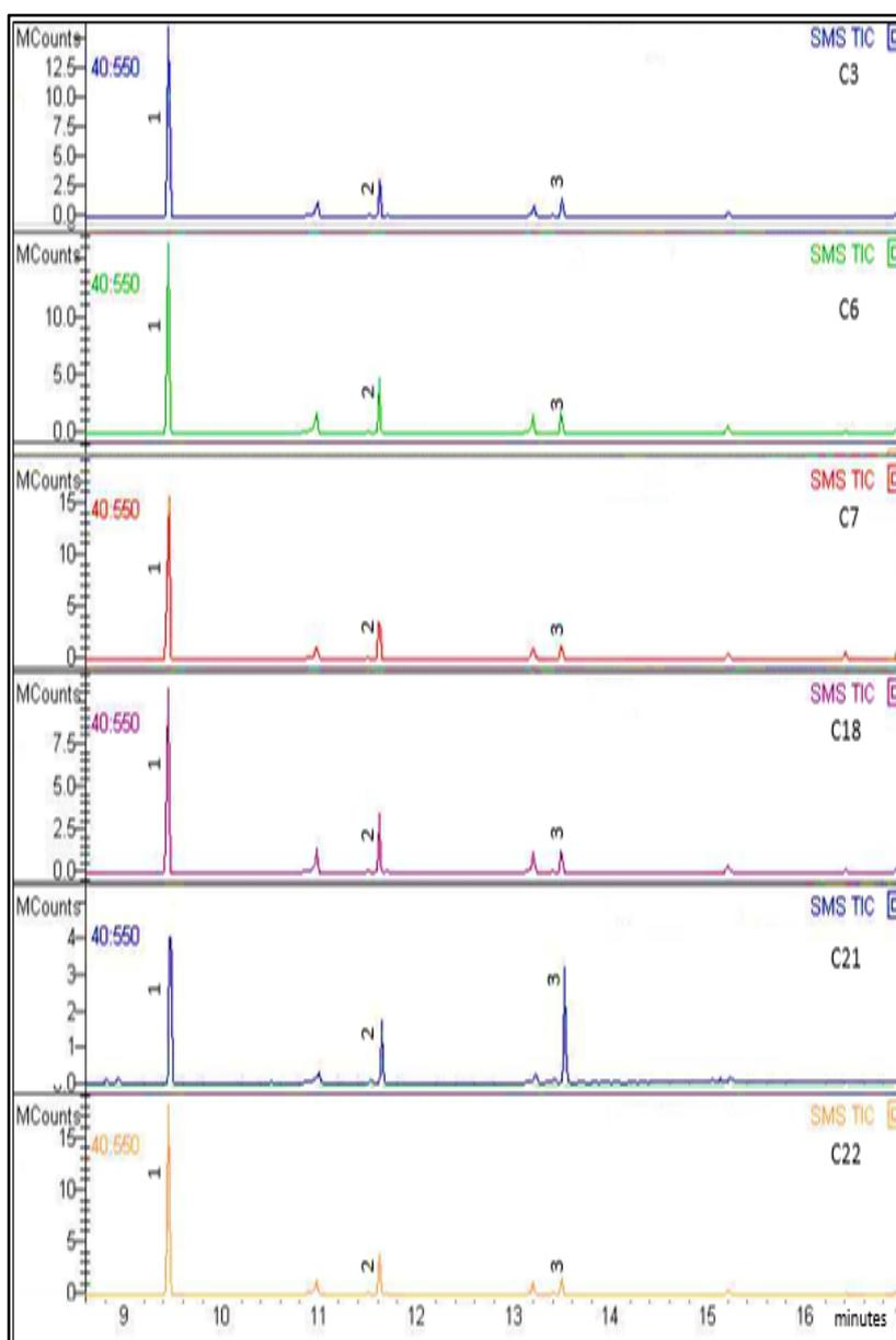
**Figure 5.** (Colour online) Secondary screening of isolates, from biodegradation assays showing chromatographic separation of organotin species and further demonstrating TBT (peak 3) degradation to DBT (peak 2) and MBT (peak 1) on day 21, detector response (y-axis) against retention time (x-axis)
