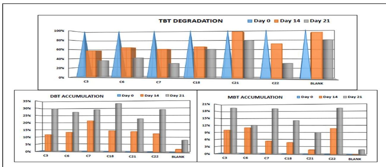
**Figure 6.** (Colour online) (Pyramid Day 0, Box Day 14, Cylinder Day 21) (Top), percentage TBT removal by isolates C3, C6, C7, C18, C21, and C22 over 21 days in cultivated MM broths (initial TBT concentration  $100 \text{ mg l}^{-1}$ ), (Left) DBT (initial concentration  $0 \text{ mg l}^{-1}$ ) accumulation over 21 days, (Right) MBT (initial concentration  $0 \text{ mg l}^{-1}$ ) accumulation over 21 days
